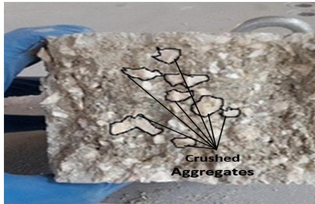
Figure 5. The transition zone in a G2 specimen.
