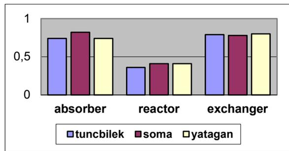
**Fig 2.** The exergetic efficiencies vs. the absorber, reactor and exchanger (tuncbilek lignite coal, soma lignite coal, yatagan lignite coal are the exergetic efficiencies
