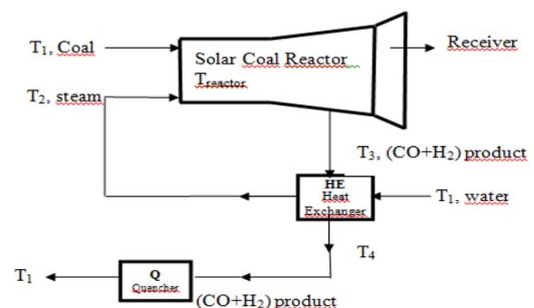
Fig 1. Solar coal gasification reactor
