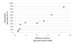
Figure 2. The variation of drying rate as a function of moisture content of pumpkin puree.
