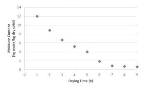
Figure 1. The variation of moisture content (db) as a function of drying time for pumpkin puree
