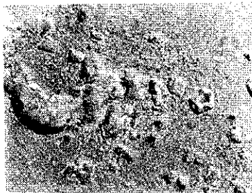
Figure 19. Photomicrograph of dispersion in Batch 5 at 100 bar, x 800
