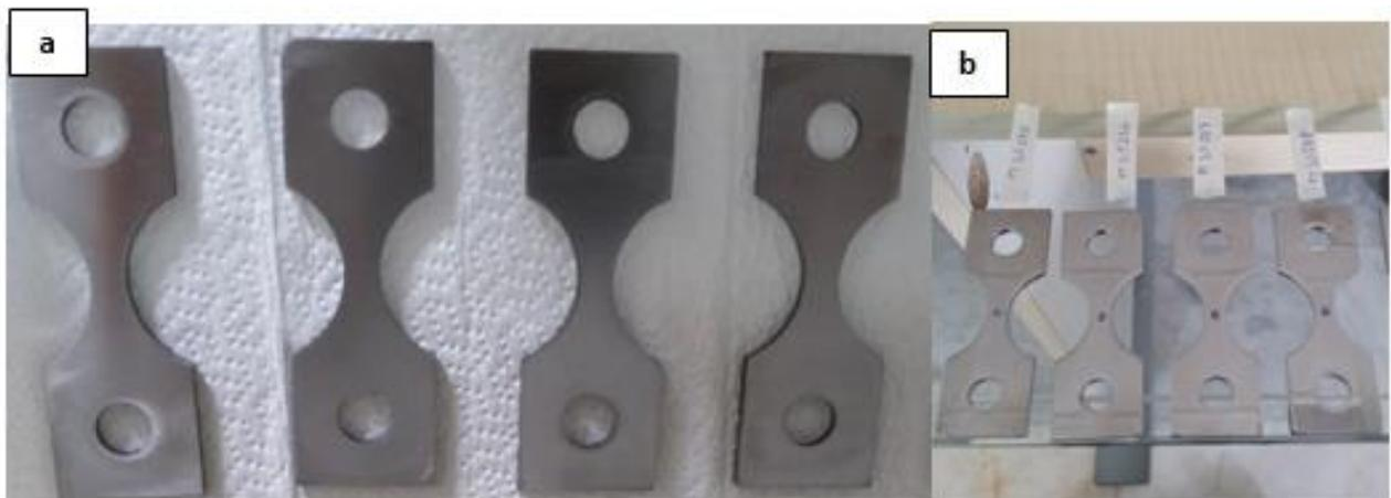
Figure 1. (a) Sanded and Ultrasonic Bathed Specimens (b) ID Numbered Specimens For 3.5 % Salinity Rate Solution
