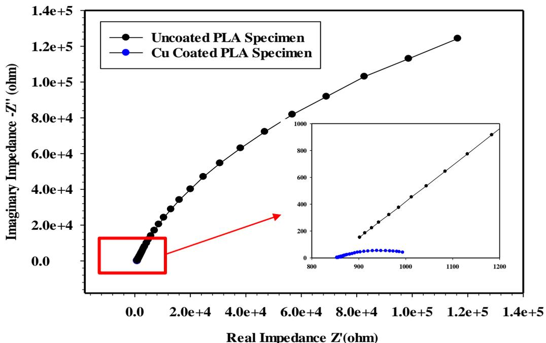
Figure 10. EIS measurements of Cu coated and uncoated PLA specimens.
