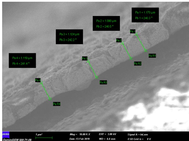
Figure 4. SEM image of the Cu coated PLA specimen electrode.
