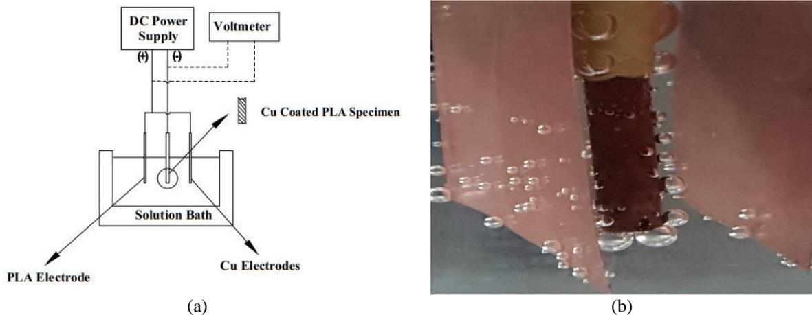
**Figure 1.** a) Electroplating procedure view of the PLA and Cu electrodes. b) Cu coating process in 0.5M H<sub>2</sub>SO<sub>4</sub> solution.
