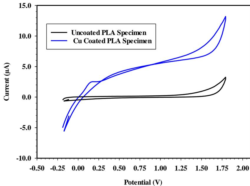
**Figure 6.** CV measurements of Cu coated and uncoated PLA specimens in the 50 mV.
