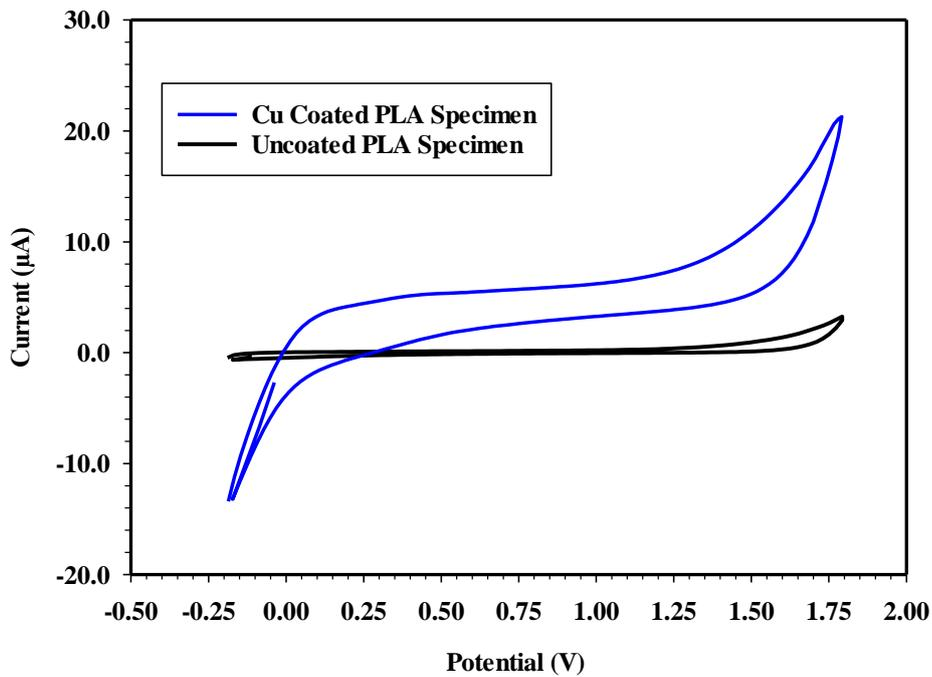
Figure 8. CV measurements of Cu coated and uncoated PLA specimens in the 200 mV.
