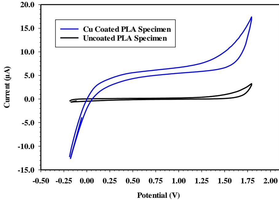
Figure 7. CV measurements of Cu coated and uncoated PLA specimens in the 100 mV.
