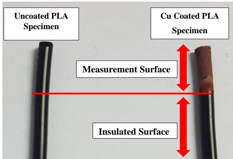
Figure 3. Uncoated and Cu coated PLA specimens.
