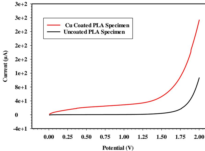
Figure 9. LSV measurements of Cu coated and uncoated PLA specimens.
