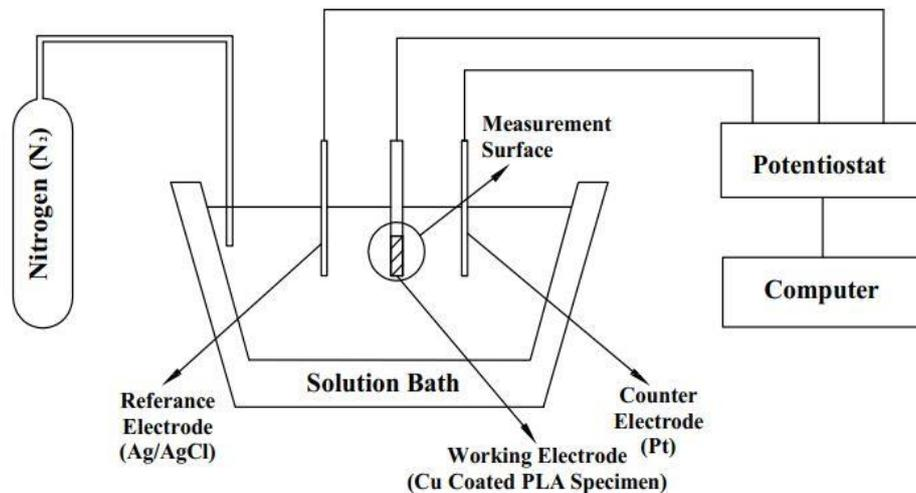
**Figure 2.** Three-electrode electrochemical cell configuration.
