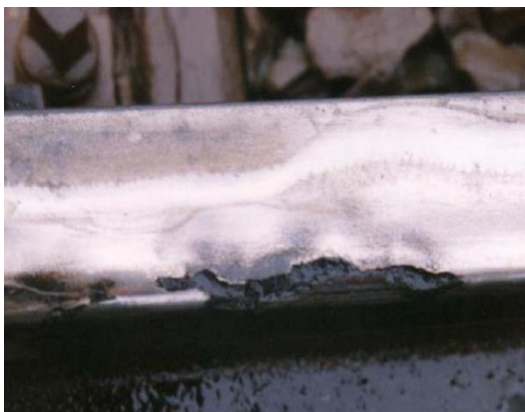
Figure 4.2. Cracks may occur on the switch
