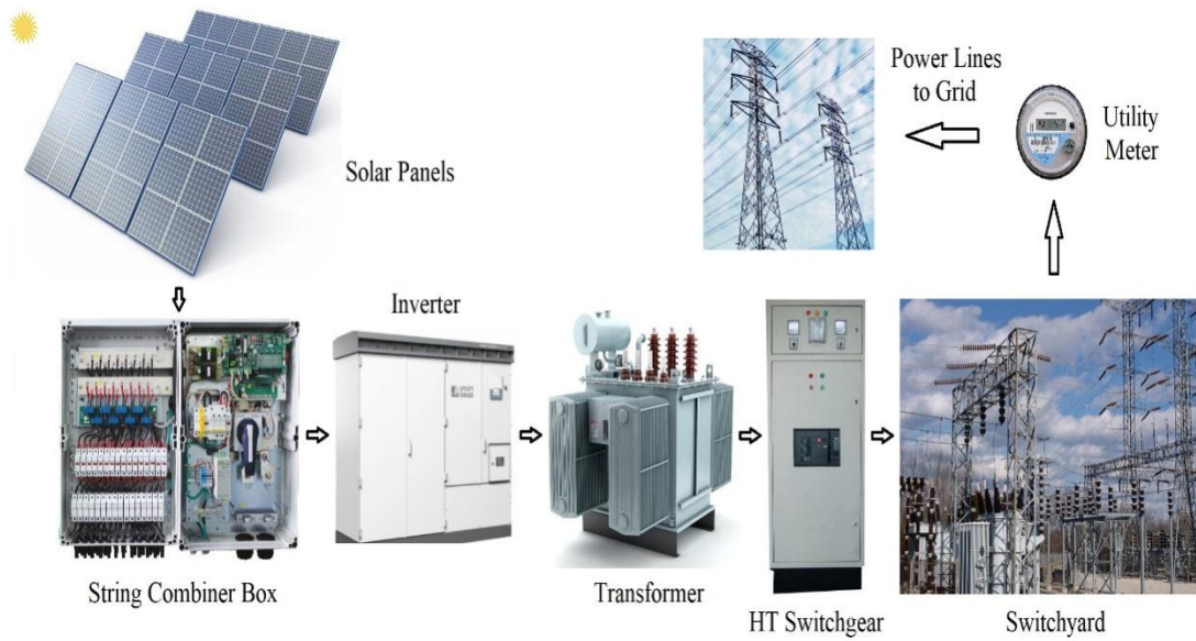
Figure 5. Schematic Diagram of the solar power plant under study
