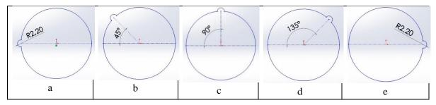
Figure 1. Positions of protrusions on the cylinder for a) 0°, b) 45°, c) 90°, d) 135°, e) 180°
