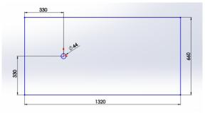
Figure 2. The schematic of the flow field (mm)
