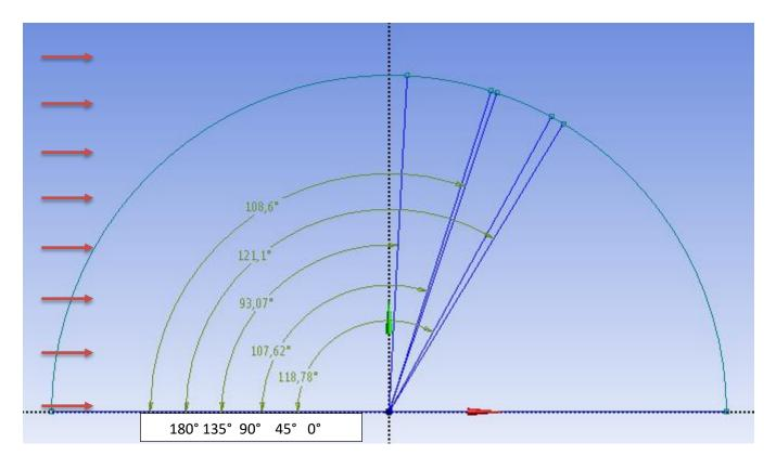
Figure 7. The angular position of separation points
