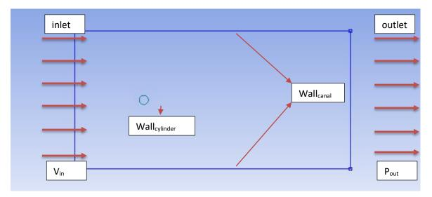
Figure 4. The boundary conditions of the flow fields
