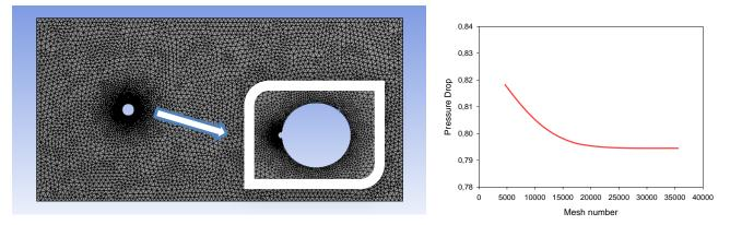
Figure 3. Mesh structure and independence
