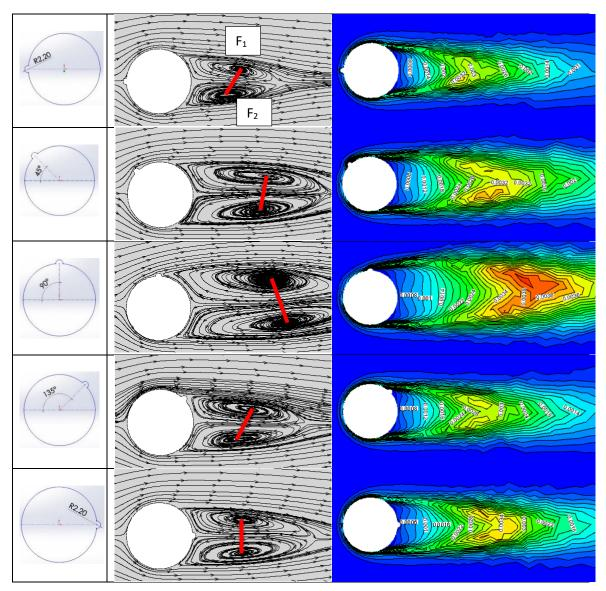
Figure 6. Streamlines and TKE contours of the models
