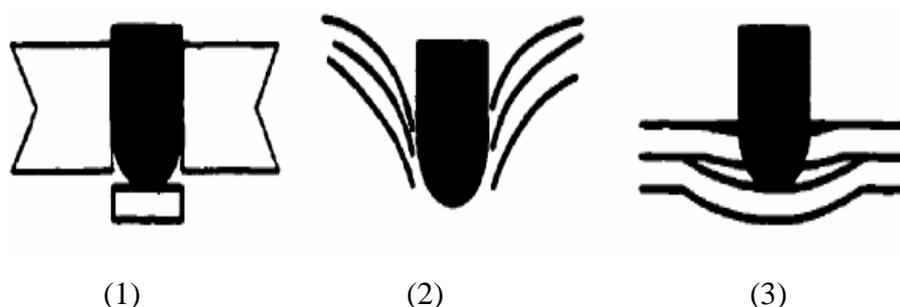
**Figure 1.** The types of ballistic impact (1) Delamination
