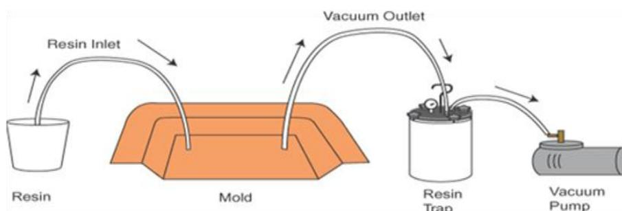
**Figure 2.** The vacuum infusion process main elements [20]
