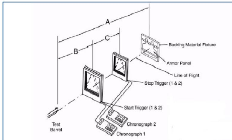
**Figure 5.** Ballistic experiment setup
