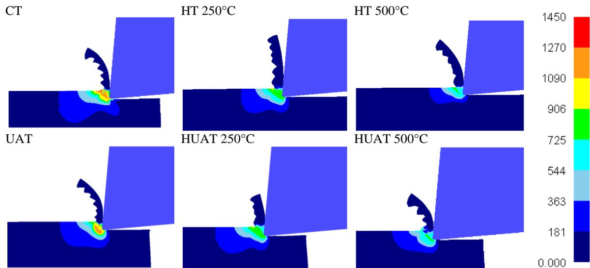
Fig. 4. Effective stresses (MPa) (Cutting speed: 30 m/min)
