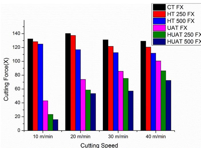
Fig. 2. Average load data for various cutting speeds
