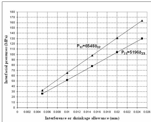
Figure 8. Interference or shrinkage allowance vs. interfacial pressure.
