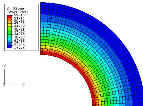
Figure 7. von Mises stress contours of holder (disk 3), MPa.
