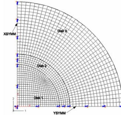
Figure 3. Finite element model of three disk shrink fit assembly.
