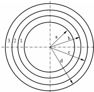
Figure 1. Three disk shrink fit assembly.
