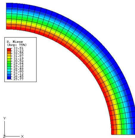
Figure 6. von Mises stress contours of sleeve (disk 2), MPa.
