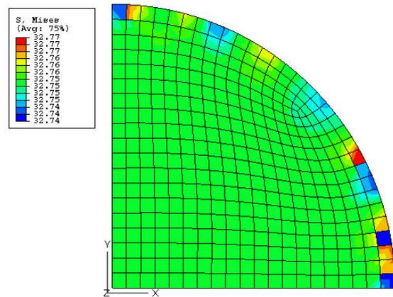
Figure 5. von Mises stress contours of solid shaft (disk 1), MPa.
