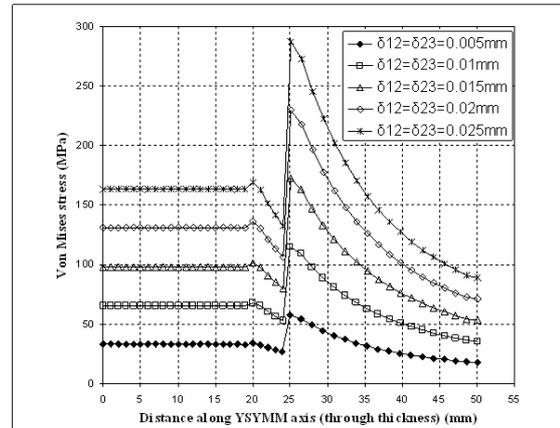
Figure 9. von Mises stress distribution along YSYMM axis (through thickness)
