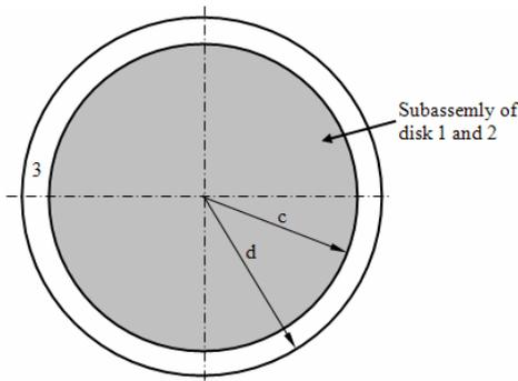
Figure 2. Final assembly of three disk shrink fit.
