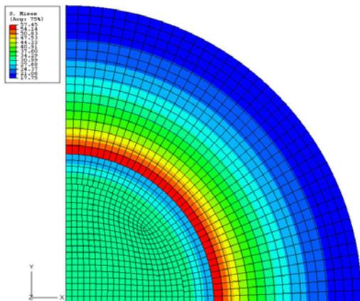
Figure 4. von Mises stress contours of three disks shrink fit assembly, MPa.
