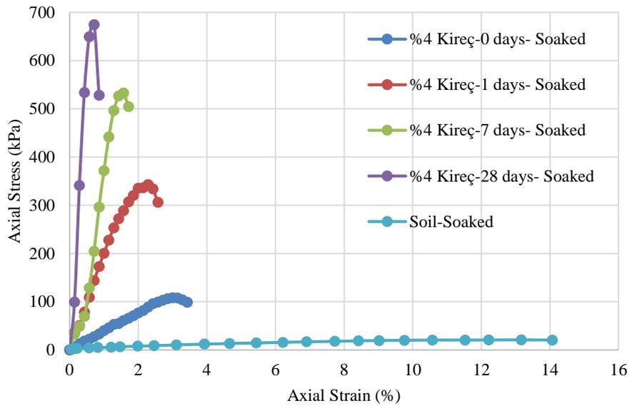
Fig. 7. Unconfined compressive strength change of soil prepared with %4 lime by weight for soaked
