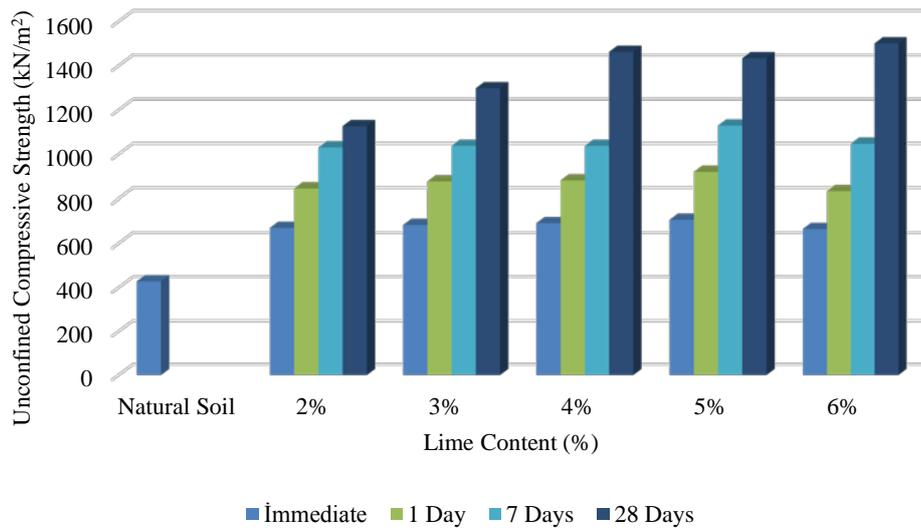
Fig. 4. Unconfined compressive strength change with curing time for different lime percentages
