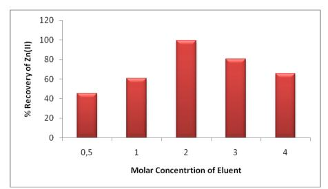
Figure 6. Effect of molar concentration of eluent on the % recovery of Zn(II)
