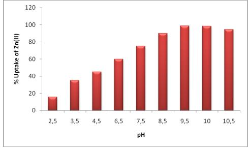
Figure 1.Effect of pH on the % uptake of Zn(II)
