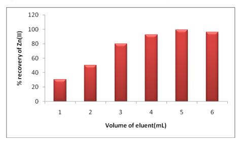
Figure 7. Effect of eluent volume on the % recovery of Zn(II)
