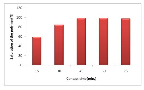
Figure 3.Effect of the contact time on the % uptake of Zn(II)
