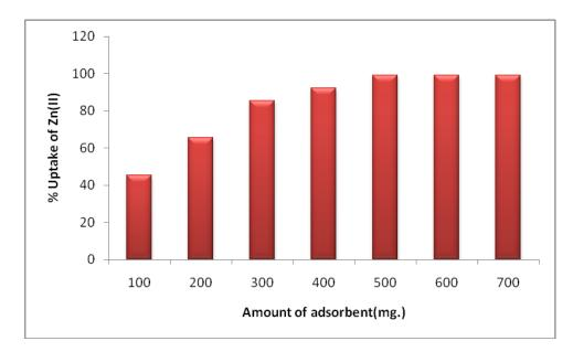
Figure 2.Effect of the amount of adsorbent on the % uptake of Zn(II)
