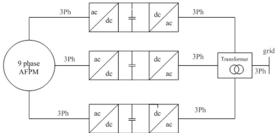
Fig.3 nine phase system configuration
