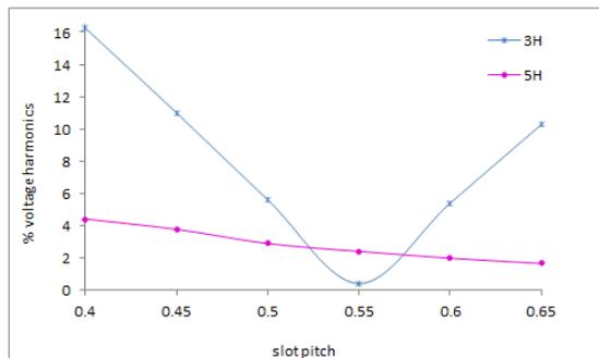
Fig.14 harmonics of no-load EMF versus slot pitch
