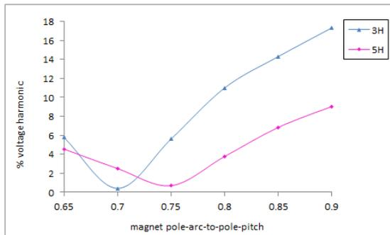
Fig.13 Harmonics of no-load EMF versus magnet pole-arc to pole-pitch ratio.
