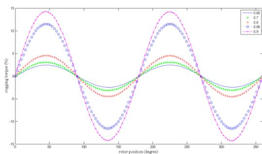
Fig.10. cogging torques at various magnet pole-arc to pole-pitch
