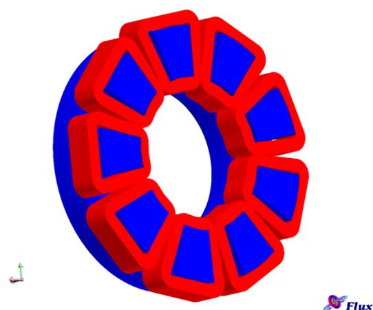
Fig.5 9-phase concentrated winding
