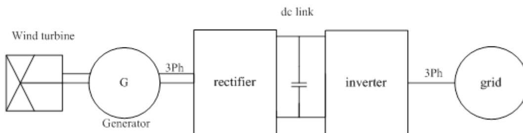
Fig.1 general schematic of wind system
