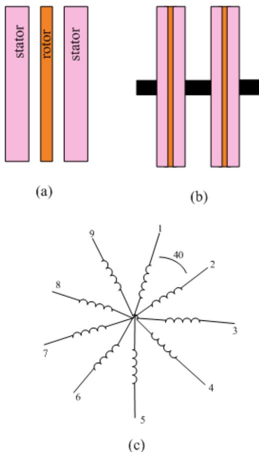
Fig.2 (a) generator structure. (b) multi-stack structure, (c) winding configuration.
