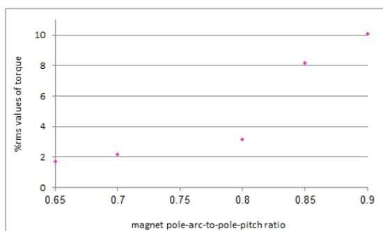
Fig.11 RMS values of cogging torque versus magnet pole-arc to pole-pitch ratio
