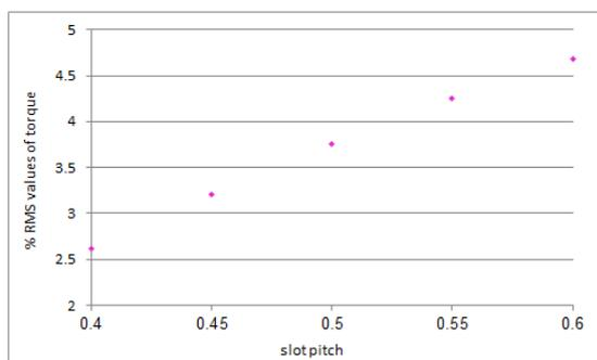
Fig.12 RMS values of cogging torque versus slot pitch
