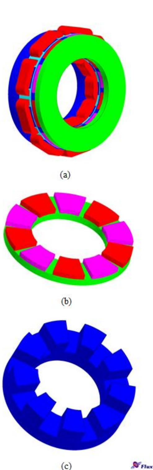
Fig.4 (a) half generator. (b) half rotor. (c) one stator
