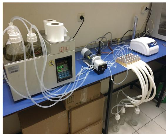
Figure 1. Drip flow reactor used in the study
