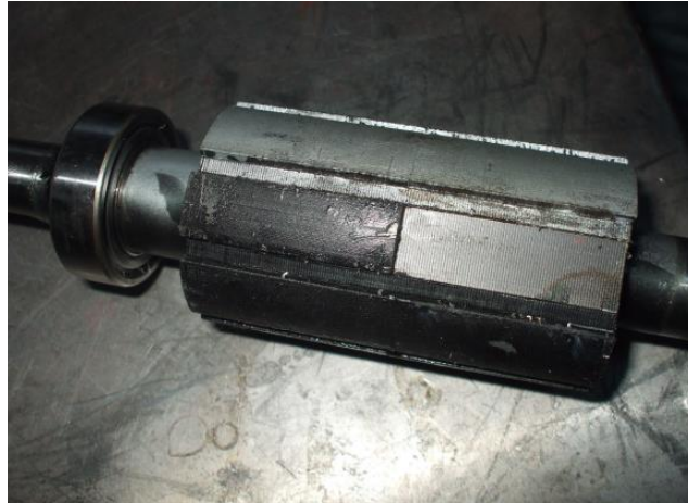
Figure 3. Used rotors (a-Healthy, b-Under 12.5% demagnetization, c-Under 18% demagnetization).
