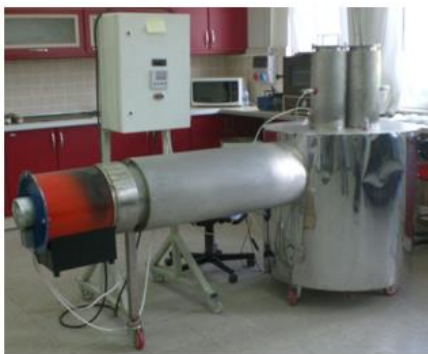
(a) (b) Figure 1. Laboratory type convective dryer (a: General view; b: Schematic view)
