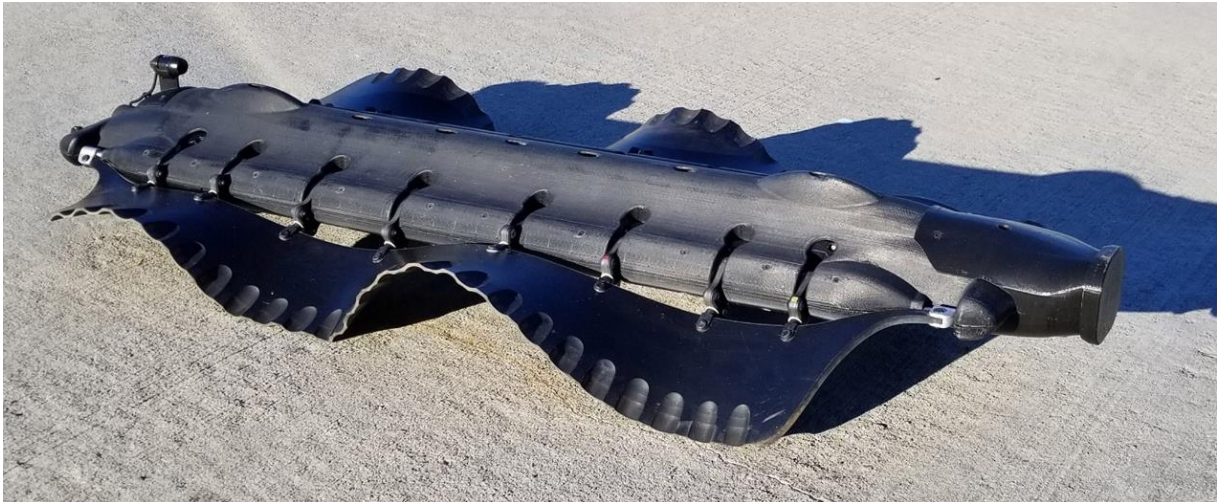
Figure 1. An amphibious robot propelled by undulating fins [18].
