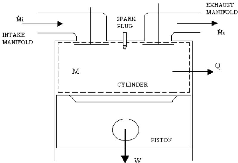
Figure 3. Engine Cylinder Thermodynamic System.
