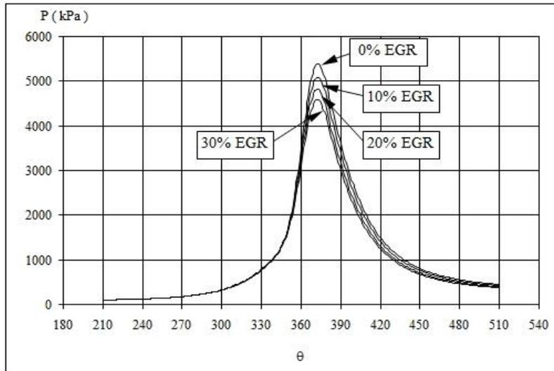
**Figure 6.** Cylinder Pressure for various percentage of EGR.
