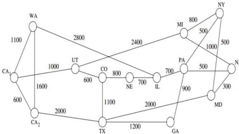
**Figure 3.** The 14-node NSFNET network topology showing approximate distances between the nodes in km.
