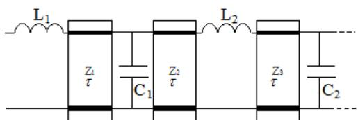
Fig. 1 Mixed-element low-pass structure (LPLU) [9]
