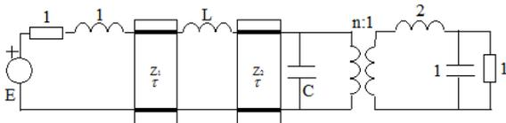
Fig. 2 Designed mixed-element matching network; proposed:
