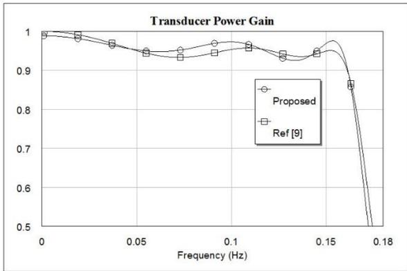
Fig. 3 The performance of the designed matching network with mixed-elements.
