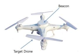
Figure 2 Beacon system design on the Phantom 4 Pro
