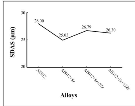
Figure 4. SDAS results of LM6 alloys with modification and alloying processes applied
