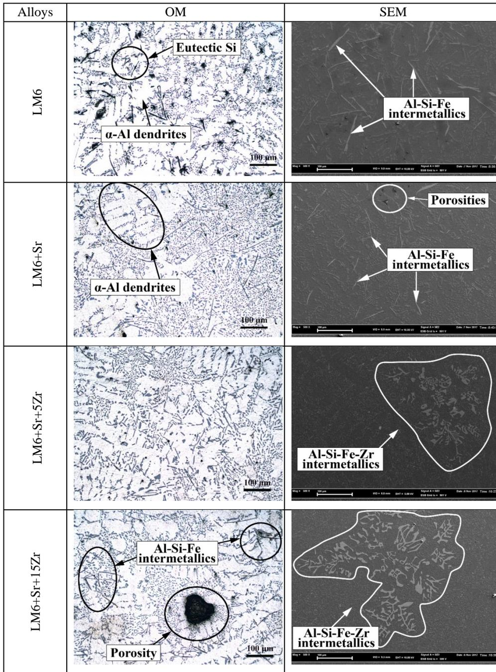
**Figure 2.** The images of optical microscope (OM) and scanning electron microscopy (SEM) of LM6 alloys which were modified and alloyed with Zr.
