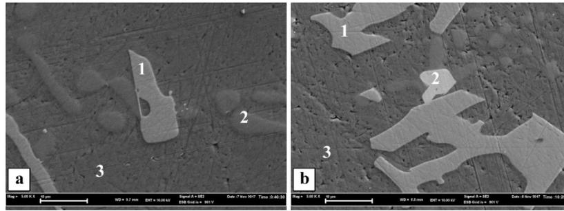
**Figure 3.** SEM images of LM6 alloys which were alloyed by 0.05% Zr (a) and 0.15% Zr.
