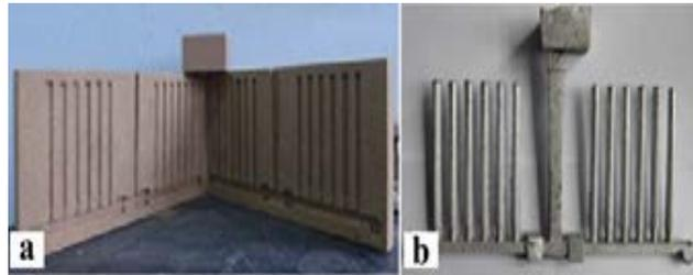
**Figure 1.** The image of sand molds (a) and image of casting parts (b)
