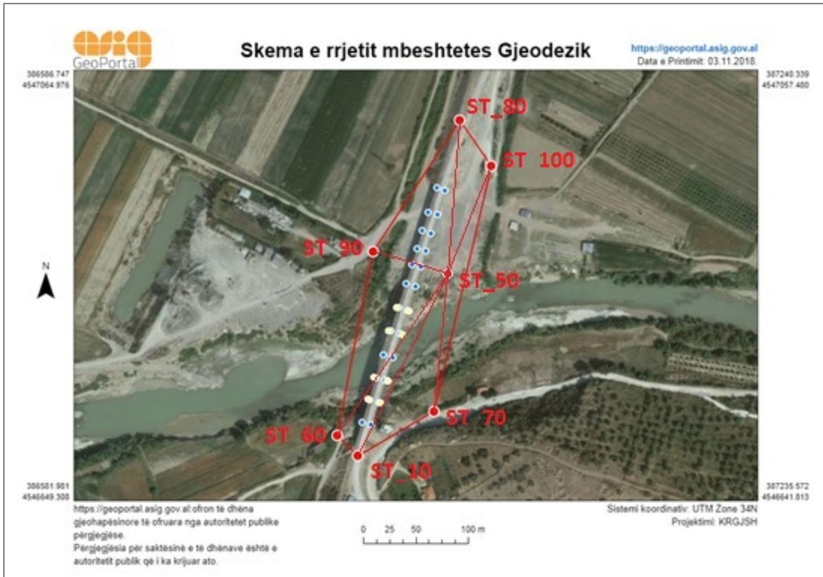
**Figure 3.** Presentation of the geodetic support network used.
