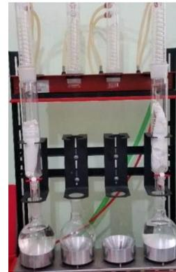
Figure 4. Soxhlet used for oil extraction
