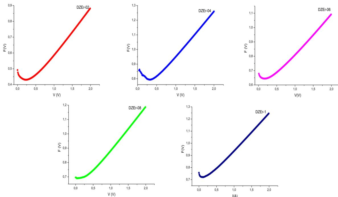
Figure 4.  $F(V)$ - $V$  plots of DZEr heterojunction diodes
