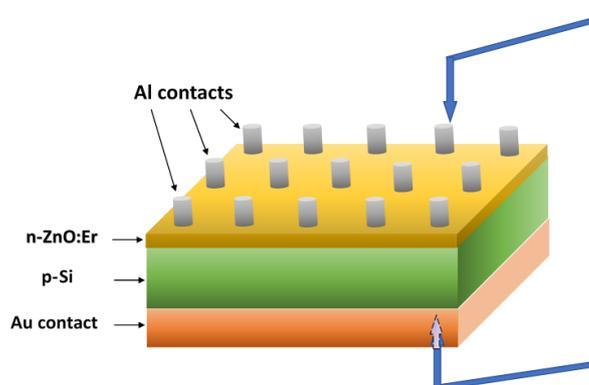
Figure 1. Schematic diagram of *p-Si/n-ZnO: Er* (DZEr) heterojunction diode
