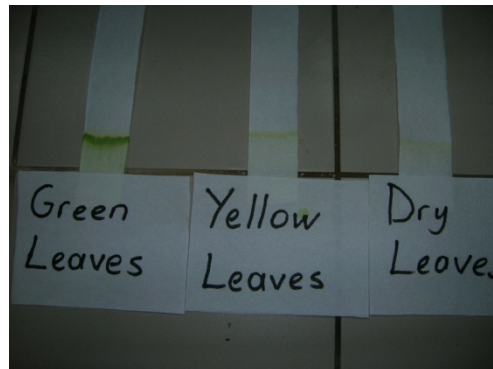
Figure 7. Results of chromatography of green, yellow and dry leaves on filter paper
