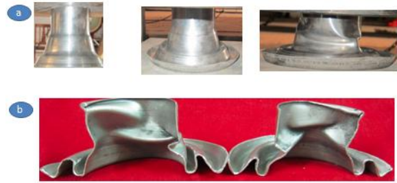
Figure 14: Deformation pattern of ST2 a) Deformation stages b) Cut sections after deformation
