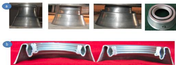
Figure 12: Deformation pattern of ST1 a) Full model at different deformation stages b) Cut sections after deformation
