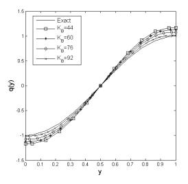
FIGURE 2. Grid Independence of the study for  $\lambda = 10^{-6}$ ,  $Ra = 10^2$ ,  $\phi = 0.05$  and  $\rho = 0$  for Case I.
