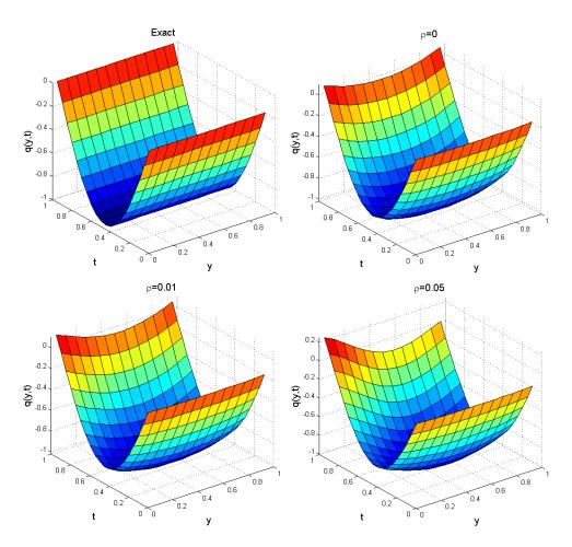
FIGURE 15. Effect of the percentage of the noise  $\rho$  on the global heat flux for  $Ra = 10^3$ ,  $\phi = 0.05$  and  $\lambda = 10^{-6}$  for Case II.
