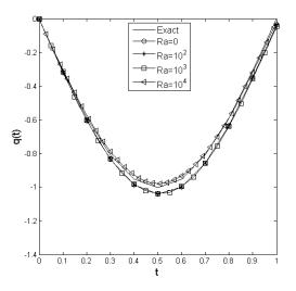
FIGURE 8. Variation of heat flux q(t) at y = 0.5 for several values of Ra when  $\lambda = 10^{-6}$ ,  $\phi = 0.05$  and  $\rho = 0$  for Case II.
