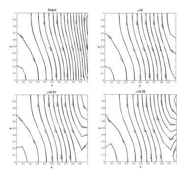
FIGURE 16. Effect of the percentage of the noise  $\rho$  on the Temperature T for  $Ra = 10^3$ ,  $\phi = 0.05$  and  $\lambda = 10^{-6}$  for Case II.
