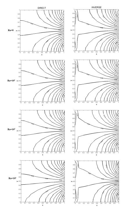
FIGURE 6. Variation of temparature for several values of Ra when  $\lambda=10^{-6},~\phi=0.05$  and  $\rho=0$  for Case I.
