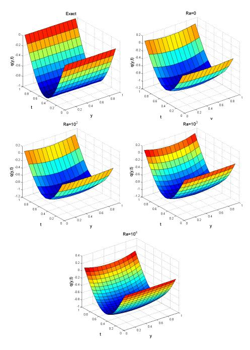
FIGURE 9. Variation of global heat flux for several values of Ra when  $\lambda=10^{-6},\,\phi=0.05$  and  $\rho=0$  for Case II.
