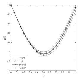
FIGURE 14. Effect of the percentage of the noise  $\rho$  on the heat flux q(t) at y = 0.5 for  $Ra = 10^3$ ,  $\phi = 0.05$  and  $\lambda = 10^{-6}$  for Case II.
