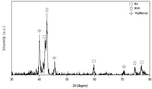
Figure 5. XRD pattern of NiTi-20Cu SMA.
