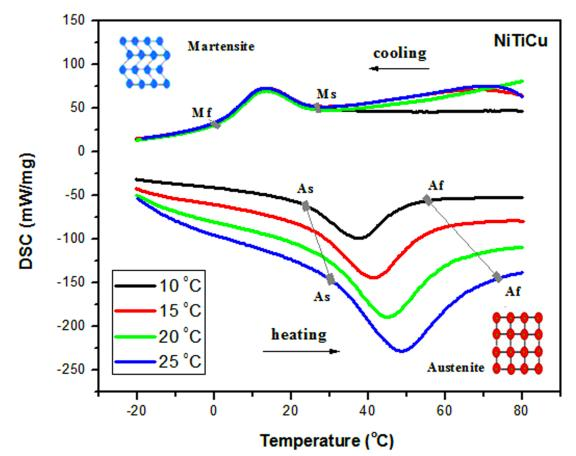
**Figure 1.** DSC curves of  $Ni_{30}Ti_{50}Cu_{20}$  alloy obtained with different heating-cooling rate.
