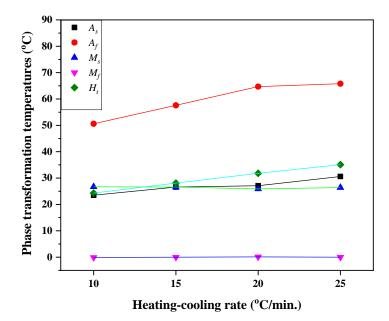
Figure 2. Change of transformation temperatures and transformation hysteresis of Ni<sub>30</sub>Ti<sub>50</sub>Cu<sub>20</sub> SMA for different heating-cooling rate
