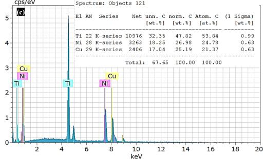
Figure 4. a) Optic micrograph, b) SEM image, and c) EDX results of NiTi-20Cu SMA
