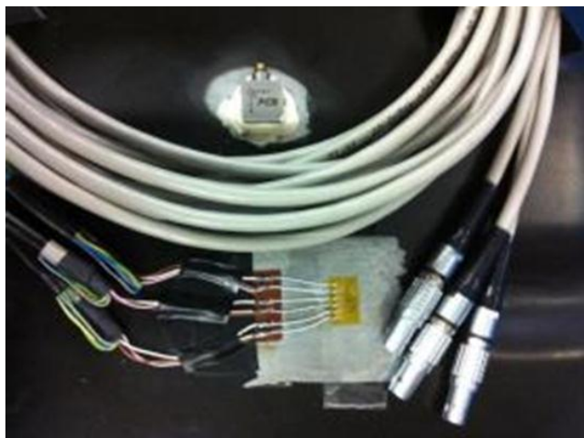
Fig. 3. Accelerometer & Strain-gage Instrumentation on the Oil Pan
