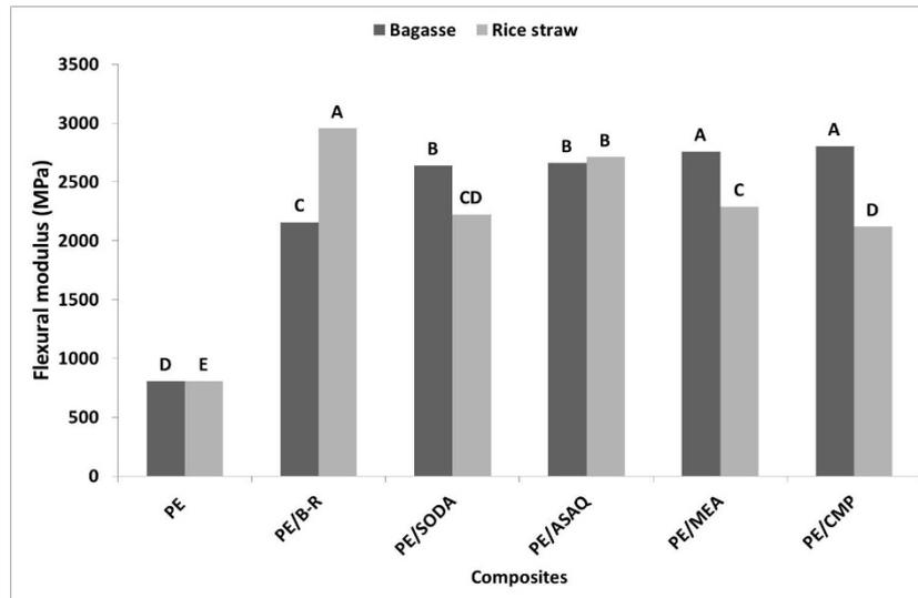
Figure 2a. Flexural modulus as function of bagasse and rice straw pulps
