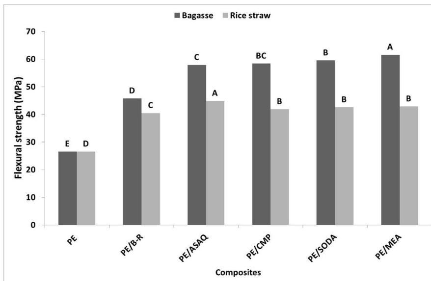
Figure 2b. Flexural strength as function of bagasse and rice straw pulps
