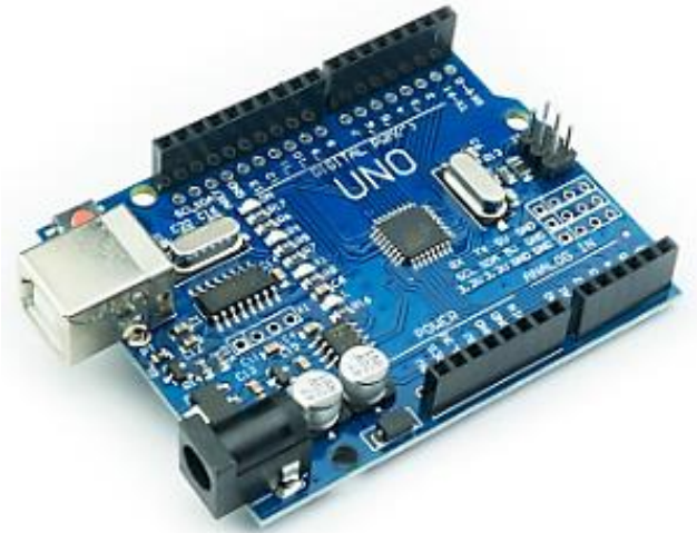
Figure 2. Arduino Uno R3 microcontroller (Anonymous, 2019)
