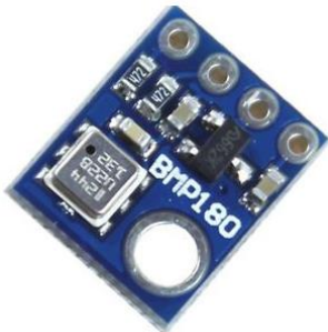
Figure 4. Digital barometric pressure sensor (Anonymous, 2019)
