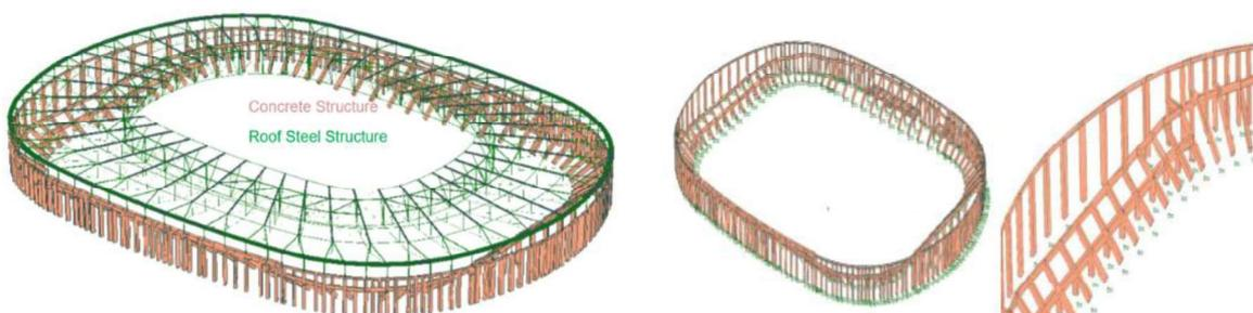
Figure 22. Concrete finite element model.
