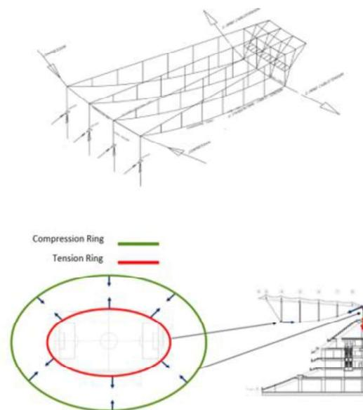
**Figure 6.** Typical load flow of besiktas stadium structural system.
