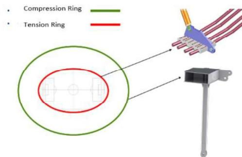
Figure 7. Tension and compression rings.
