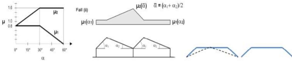
Figure 11. Snow loads on the roof.
