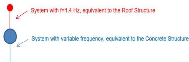
**Figure 24.** Concrete-Roof structure system frequencies.
