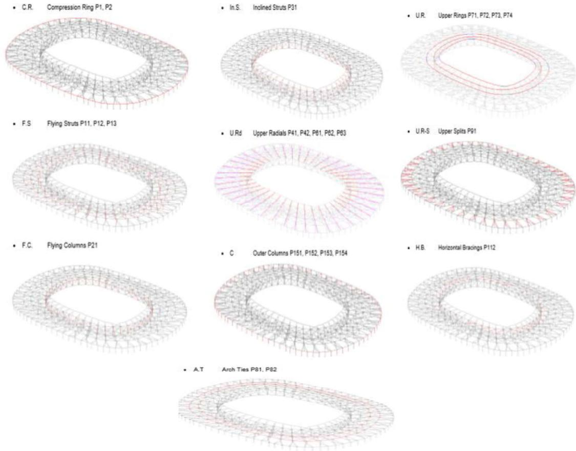
Figure 8. Steel frame elements.
