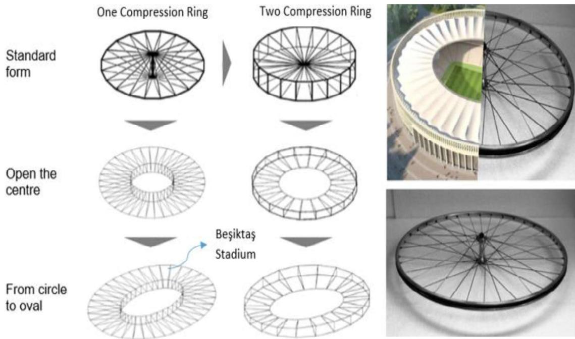
Figure 7. Typical bicycle wheel carrier system applications.
