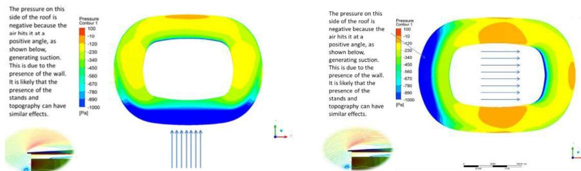
Figure 18. Stress contours on the roof.
