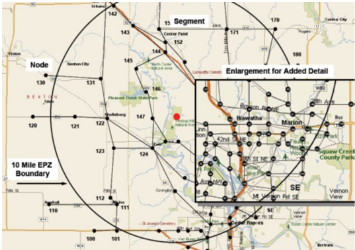
Figure 2. Sample Roadway Network Map Identifying Nodes and Segments (U.S. NRC, 2011)
