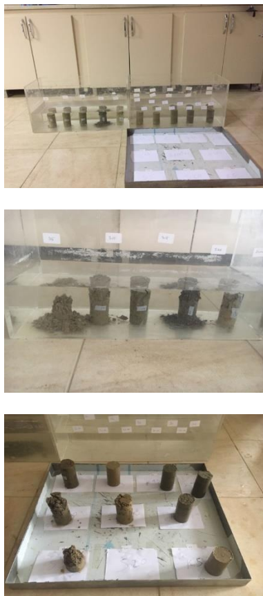
Figure 7. Illustration of wetting-drying cycle
