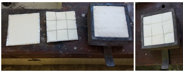
Figure 1. Sample preparation and retaining grid geometry.
