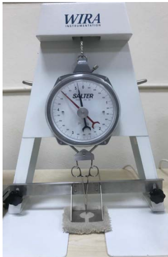
Figure 1. Pile withdrawal test device.
