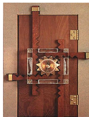
Figure 16. A lock model of four bolted case door (Sezgin, 2003).
