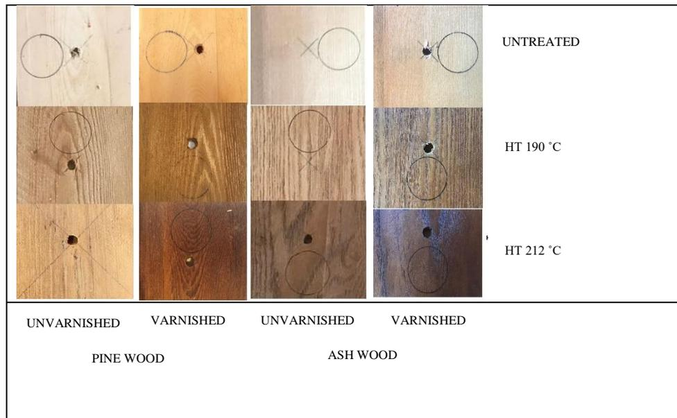
**Figure 2.** The colour change caused by heat treatment process and varnish on wood samples
