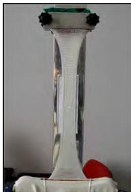
Figure 4. Special apparatus to measure the load-extension properties in this work (Elmalı [18]).
