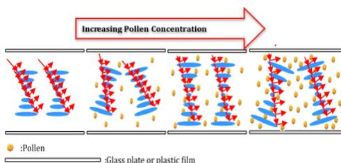
**Figure 5.** Schematic representation of the change in helical pitch of ChLC doped with pollen.
