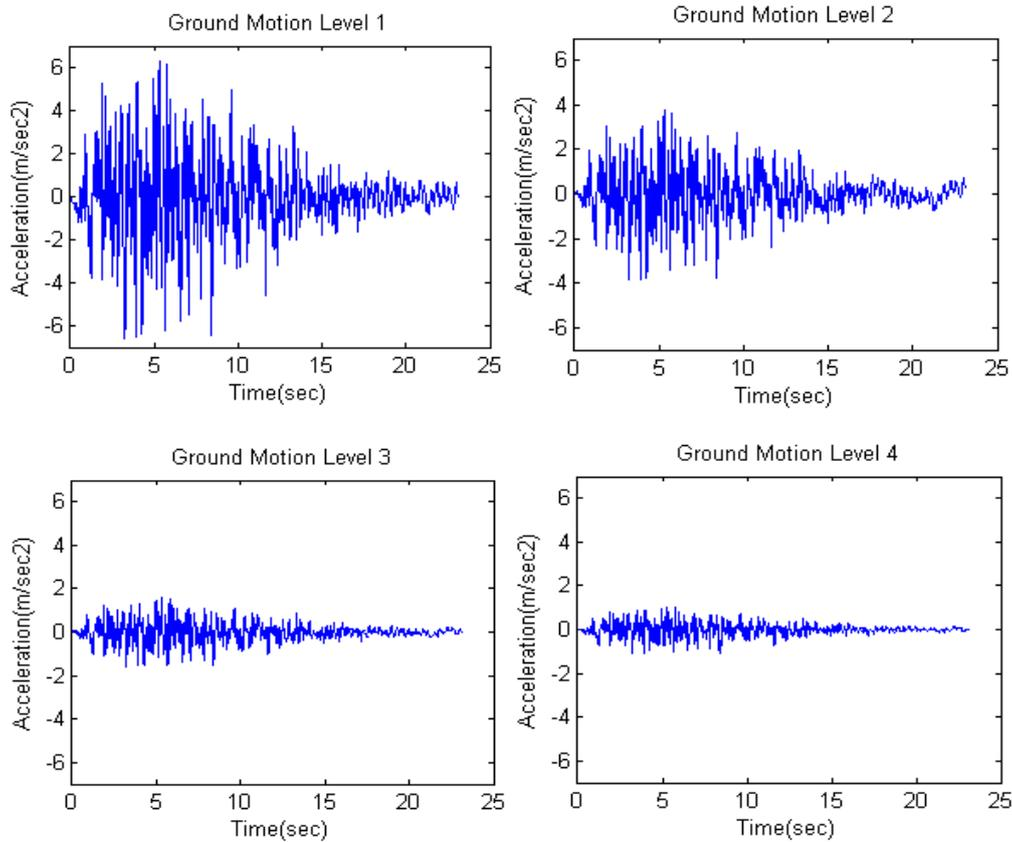
**Figure 5.** Acceleration time histories of the synthetic ground motion for four ground motion level
