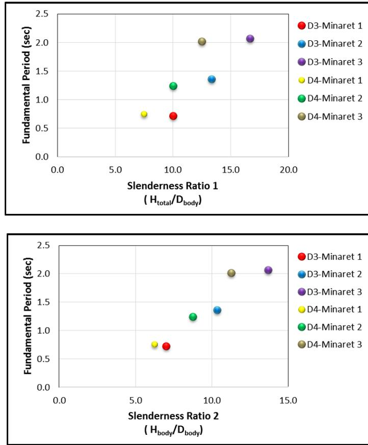
Figure 4. Variation of natural periods with respect to slenderness ratio 1,  $Sr_1$  and slenderness ratio 2,  $Sr_2$
