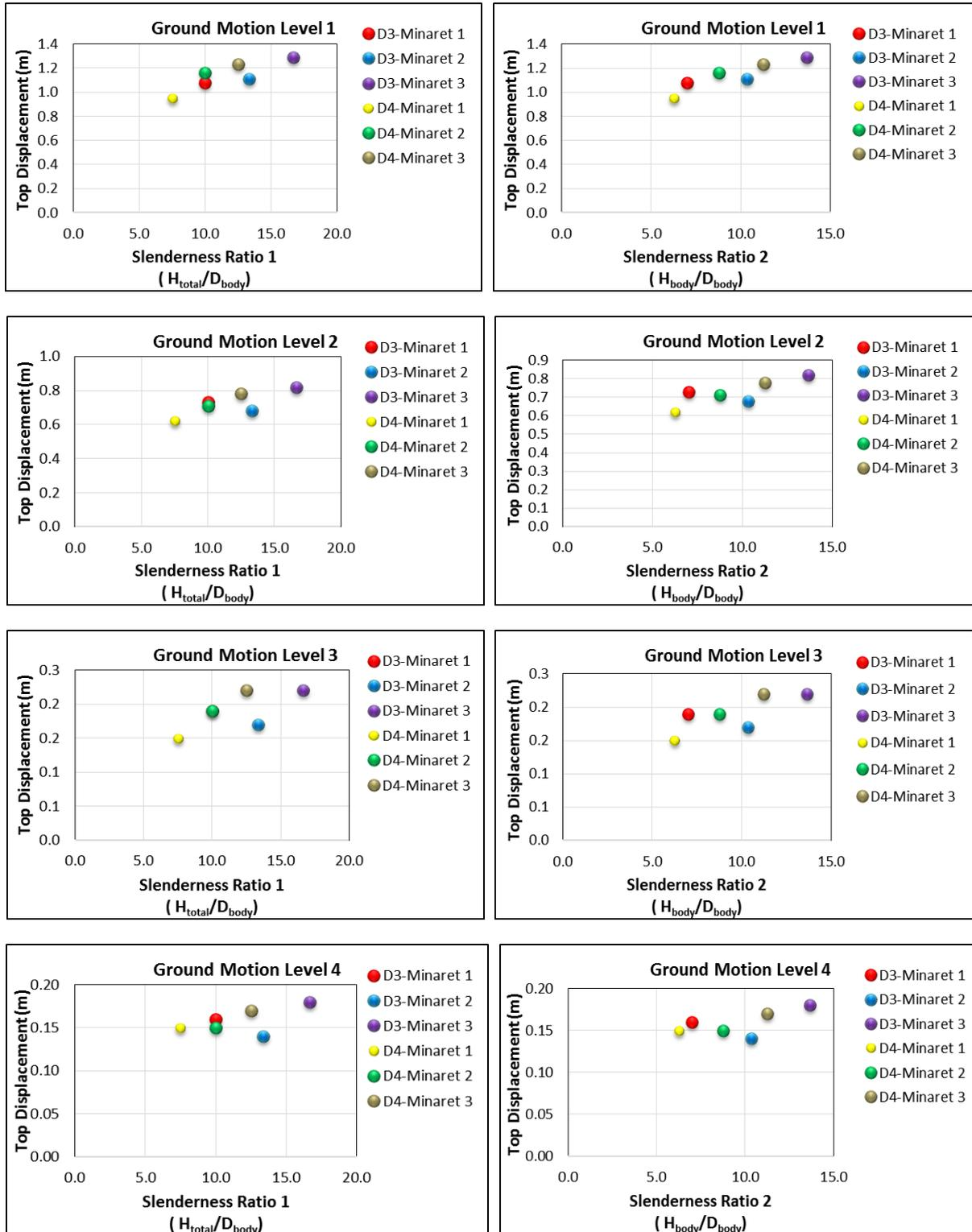
Figure 6. Variation of top displacement with respect to slenderness ratio 1, Sr1 and slenderness ratio 2, Sr2 for four ground motion level
