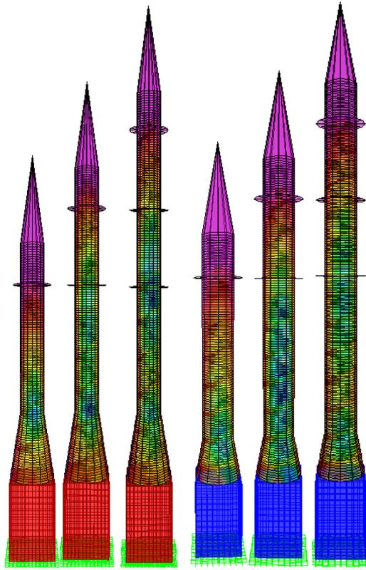
**Figure 8.** Variation of shear stresses along the first group of minarets with drum diameter of 3m (a) and second group of minarets with drum diameter of 4m (b) for ground motion level 1
