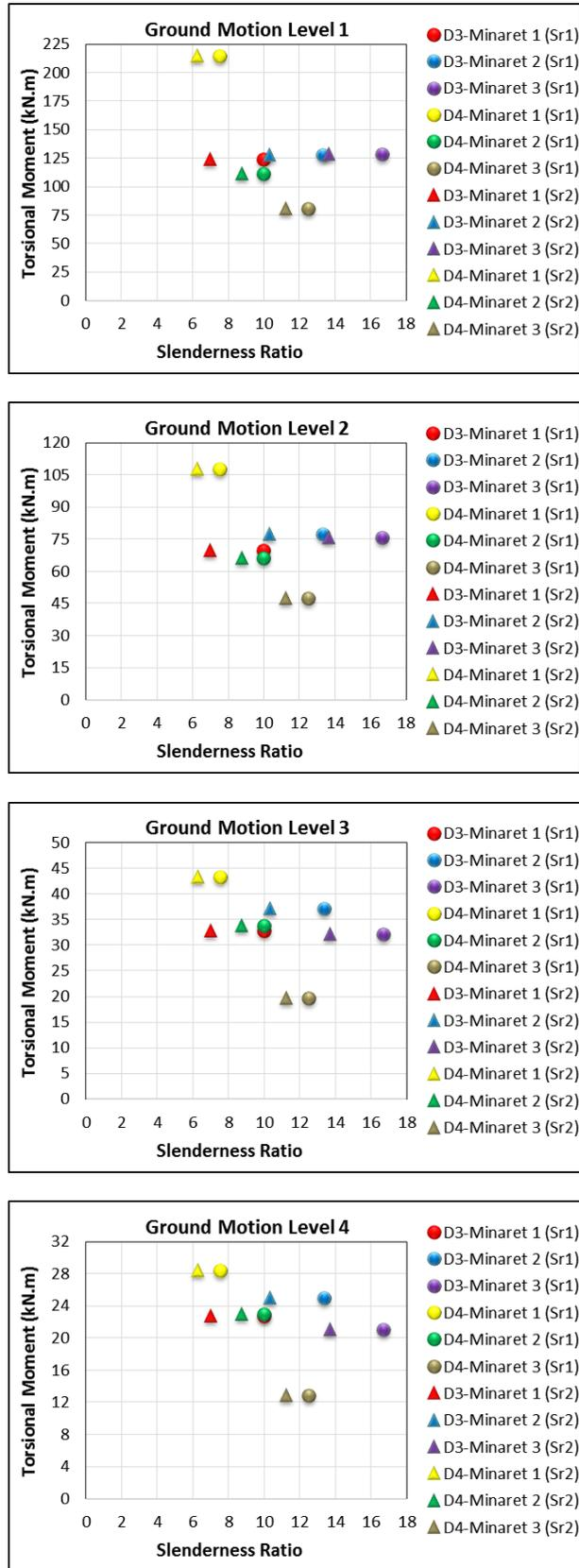
Figure 7. The variation of torsional moment at the base of the minarets with respect to slenderness ratio 1,  $S_{r1}$  and slenderness ratio 2,  $S_{r2}$  for four ground motion level
