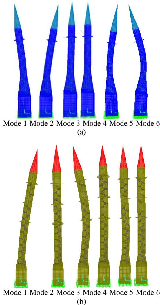
**Figure 3.** First six mode shapes of the 40 m height of the minarets with external drum diameter of 3m (a) and 60 m height of the minarets with external drum diameter of 4m (b)
