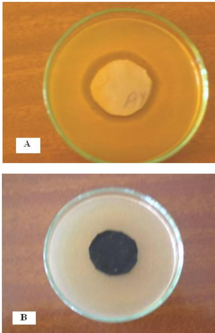
**Figure 1.** Determination of antibacterial activity by EN ISO 20645:2004 method. A: Antibacterial specimen, B: Control specimen
