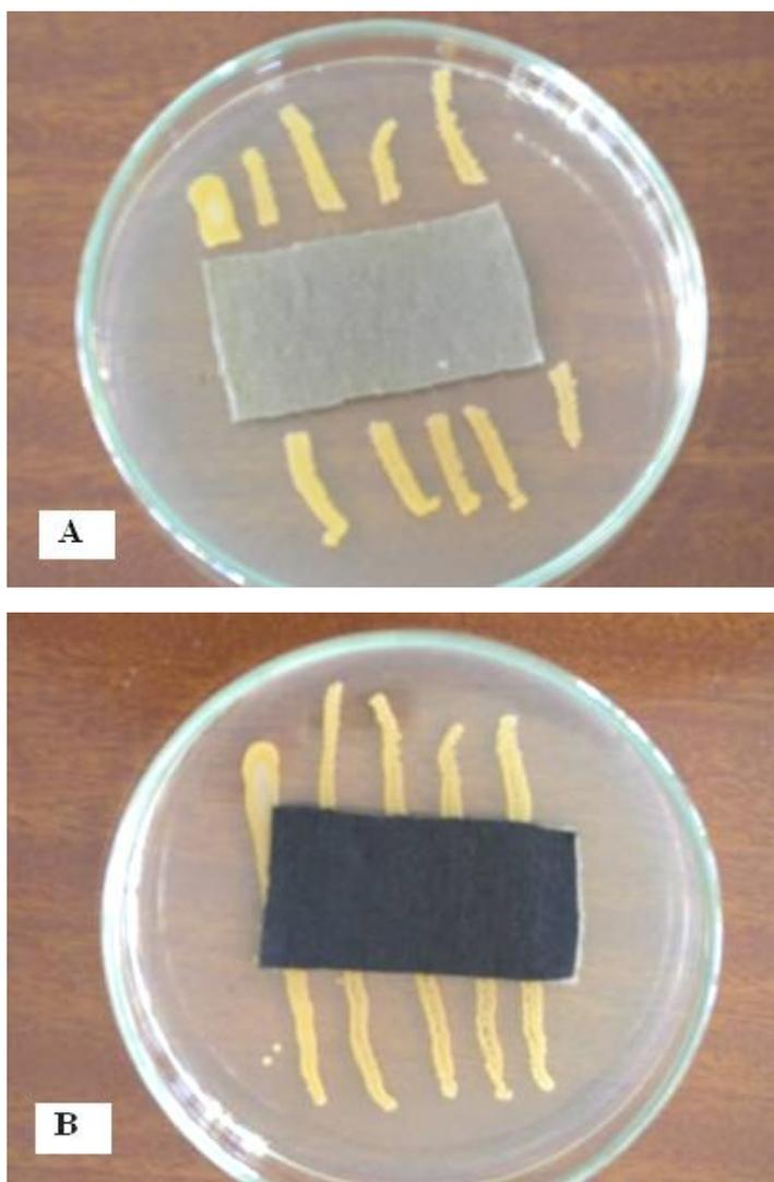
**Figure 2:** Determination of antibacterial activity by AATCC 147-2004 method. A: Antibacterial specimen, B: Control specimen.
