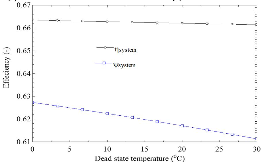
**Fig.4.** System efficiency versus with dead state temperature
