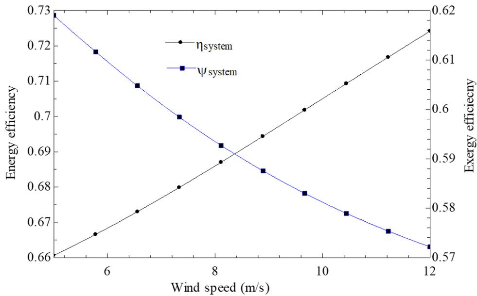
Fig.7. Influence of the wind speed on the total plant's performance
