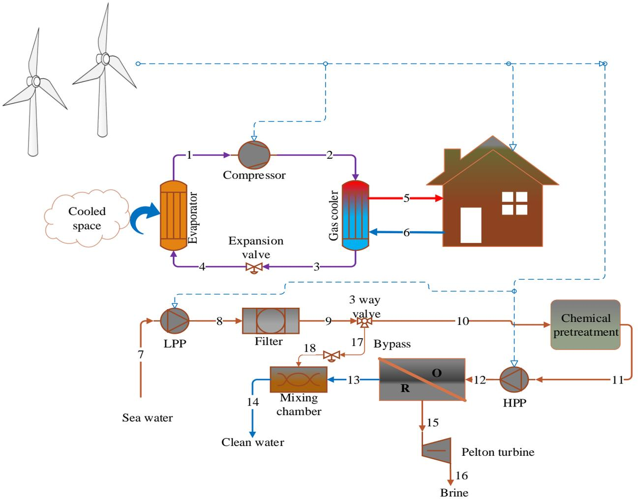
Fig.1 Schematic presentation of wind turbine combined system
