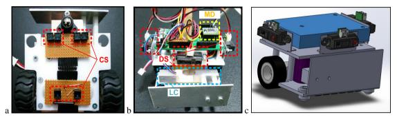
Figure 2. Implemented robot views. (a) Bottom view with the contrast sensors. (b) Top and front view with the load cell, the motor drive, and the distance sensors. (c) Solidworks drawing of the robot
