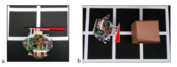
Figure 15. Main causes of errors. (a) Line deflection angle (b) Approach deflection angle
