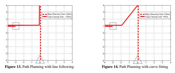
Cargo was placed at the coordinates (-3, Y) in the test setup and the travelled distance for each cargo carrying task was measured. The distances for each method are shown in Table 1. The travelled distance was reduced up to 17.5% with curve fitting method.
