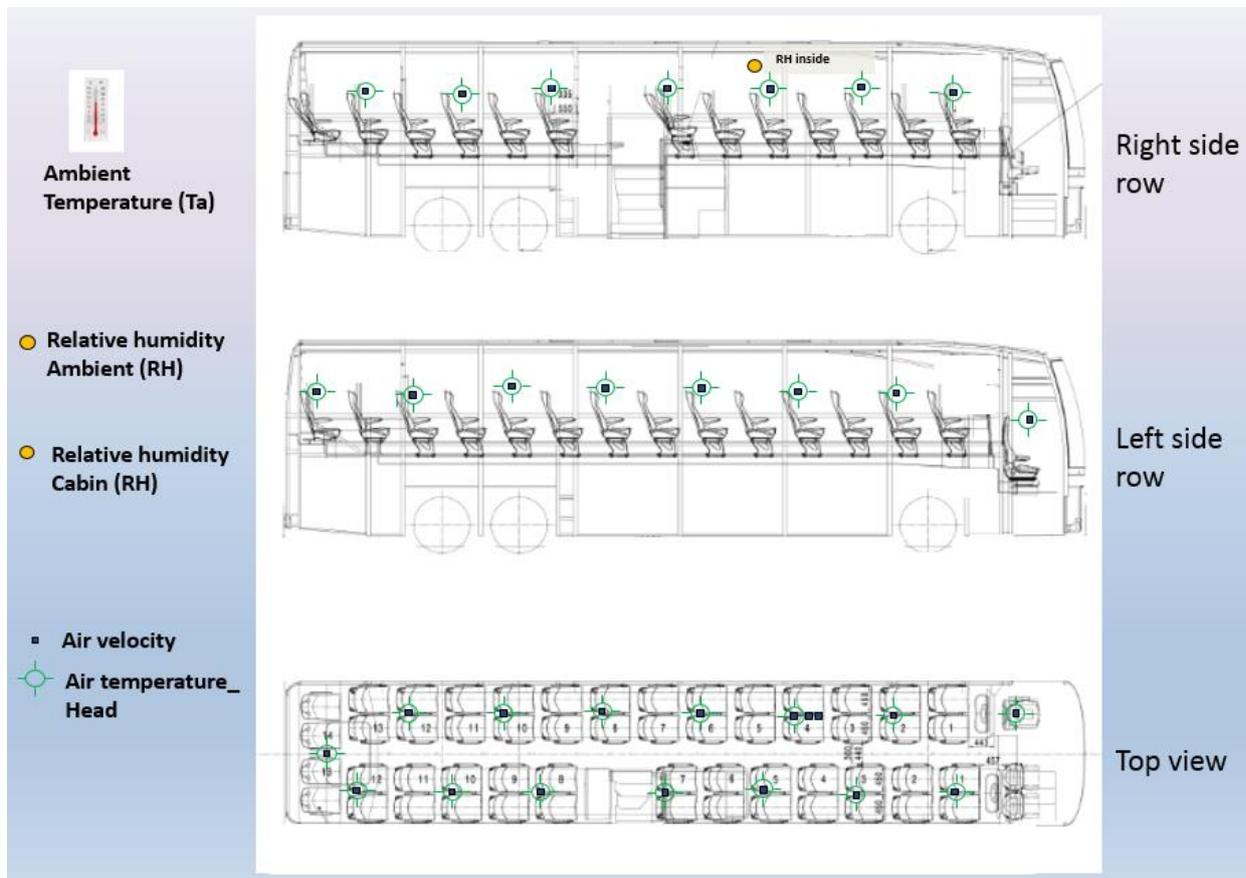
**Figure 1.** Measurement Points on the Passenger Bus
