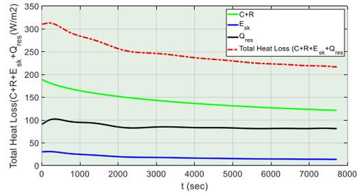
**Figure 8.** Total Heat Losses as overall (C+R+Qcd+Qres+Esk)
