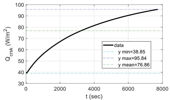
Figure 4. Heat Energy Flow between Core and Skin
