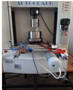
Figure 4. Biomechanical Joint Wear Simulator Test Setup
