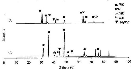
**Fig. 4** XRD results of specimens sintered at (a)  $1050^\circ\text{C}$  air atmosphere, (b)  $1050^\circ\text{C}$  Ar atmosphere
