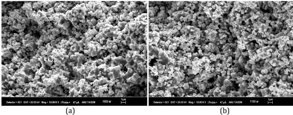
**Fig. 3** SEM images of the specimens sintered at (a)1050°C (b)1150 °C under Ar atmosphere (10.000X)
